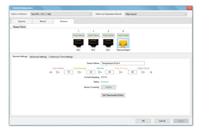
The configuration and options for the Thermal Map's sensors are the same as with standalone sensors.
