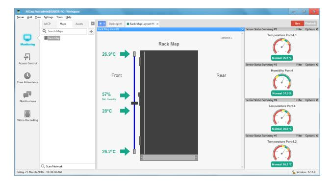
Finally, drag-and-drop the previously created Rack Map to the workspace. This will visually show all current sensor readings according to the Rack Map setup.
