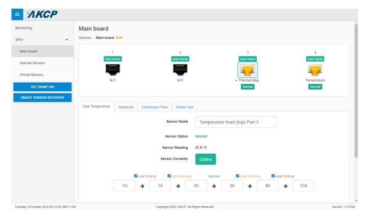
The configuration and options for the Thermal Map's sensors are the same as with standalone sensors.
