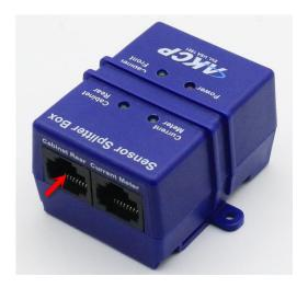
Refering to the picture above, next connect the remaining 3 sensors string to the oposite sensor port on the i2C unit labeled as "Cabinet Rear." Then these 3 sensors need to installed in the rear of your server cabinet.
