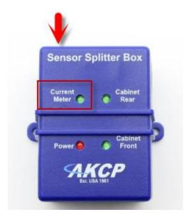
The Contactless Current Meter or CCM connects to the port located left of the Cabinet Rear port on the Splitter Box as shown above.
