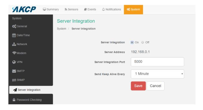
Before adding the unit to the APS console, ensure that the **Server Integration** option is **enabled** in the Web UI's **System page**.
