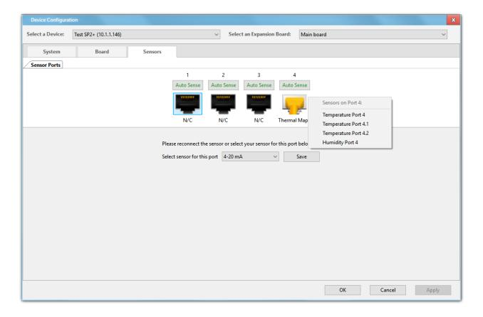
In the **Device Configuration** window, you'll see the **Thermal Map** as a single sensor.
