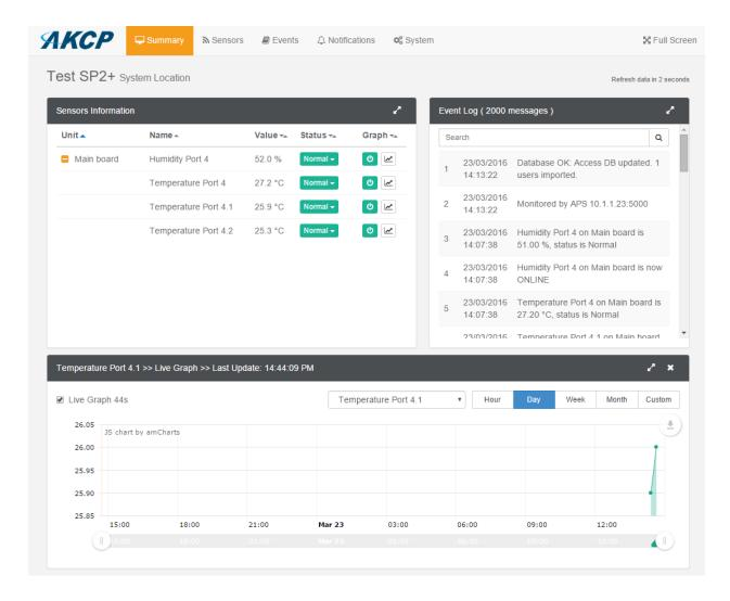
On the **Summary page** you can see the connected Thermal Map as multiple sensors. For example from the Temperature/Humidity sensor you can easily identify which port it is plugged in to on the unit (you can also freely rename the sensors afterwards).
