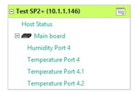
After the initialization has finished, you can see the connected Thermal Map sensor as multiple sensors, similar to the view of the unit's Summary page on the Web UI.
