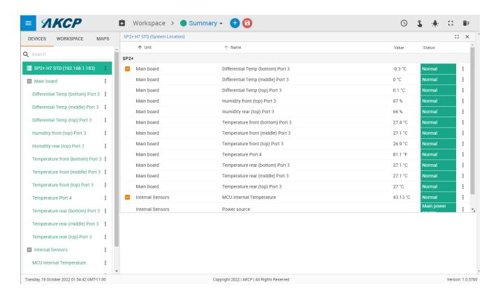
On the **Summary page** you can see the connected Thermal Map as multiple sensors. For example from the Temperature/Humidity sensor you can easily identify which port it is plugged in
