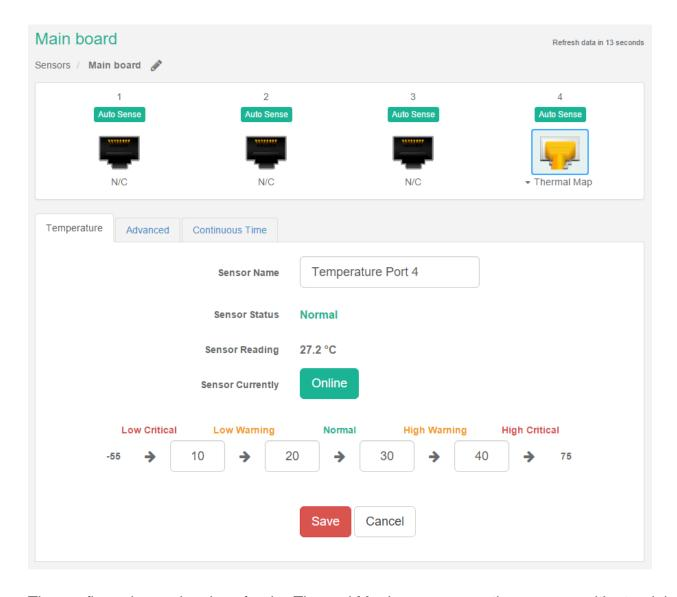
The configuration and options for the Thermal Map's sensors are the same as with standalone sensors.
